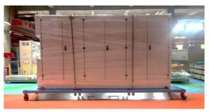
• For irregular parts like external protective shells, large castings, and shafts, custom fixtures and transport tools are used, but become unusable with product changes and can't be stacked, wasting space. Microone's solution uses standard pallets with minimal custom supports. When products change, only supports need replacement, allowing continued use of pallets, reducing costs. Standard pallets can be stacked, and custom supports stored separately, saving space. Here's a reference case.
